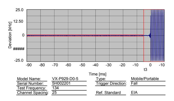
NAME OF TEST: Transient Frequency Behaviour
