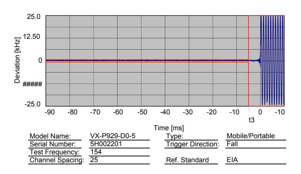
NAME OF TEST: Transient Frequency Behaviour
