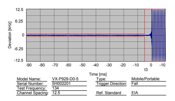
NAME OF TEST: Transient Frequency Behaviour
