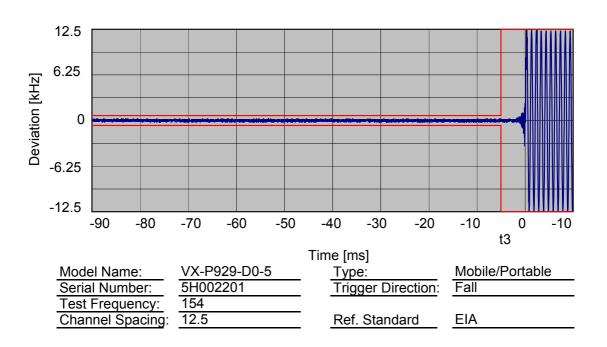
NAME OF TEST: Transient Frequency Behaviour
