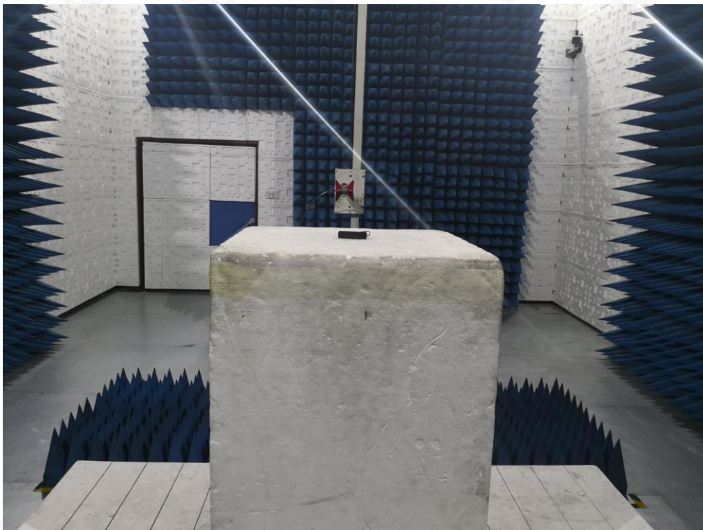
RADIATED EMISSION TEST SETUP ABOVE 1GHZ
