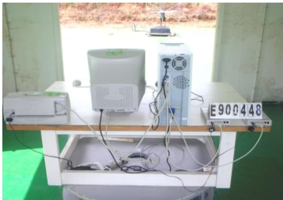
**RADIATED EMISSIONS TEST DATA****Transmitter (TX OFF)****Antenna polarization : HORIZONTAL ; Test distance : 3 m ;**
