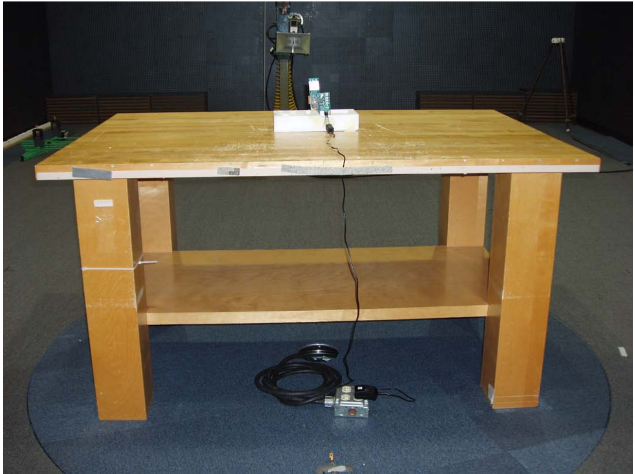
Photo 5.5-2 - Rear View of the Radiated Emissions Test Set-up
