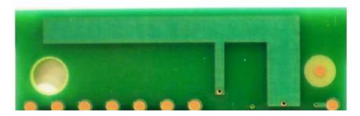
The ZIM-B module includes an integrated Printed Circuit Board (PCB) trace antenna with a nominal gain of -1.0 dBi.
