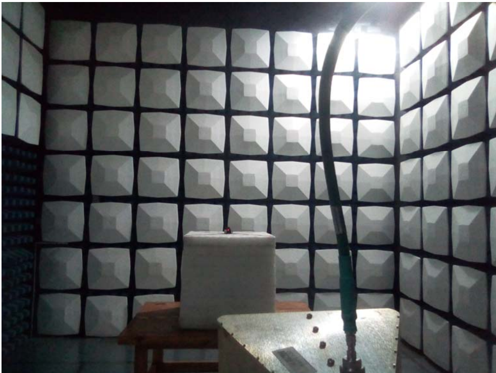
Radiated Emission 1 GHz-26.5GHz View(3m distance)
