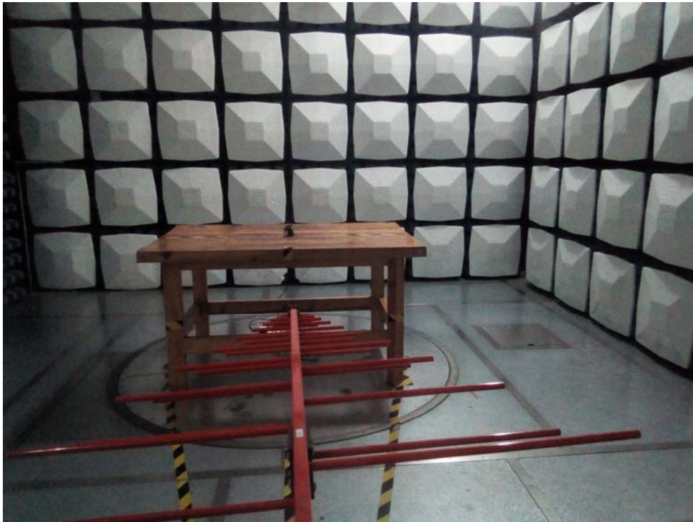
Radiated Emission 1 GHz-26.5GHz View(3m distance)
