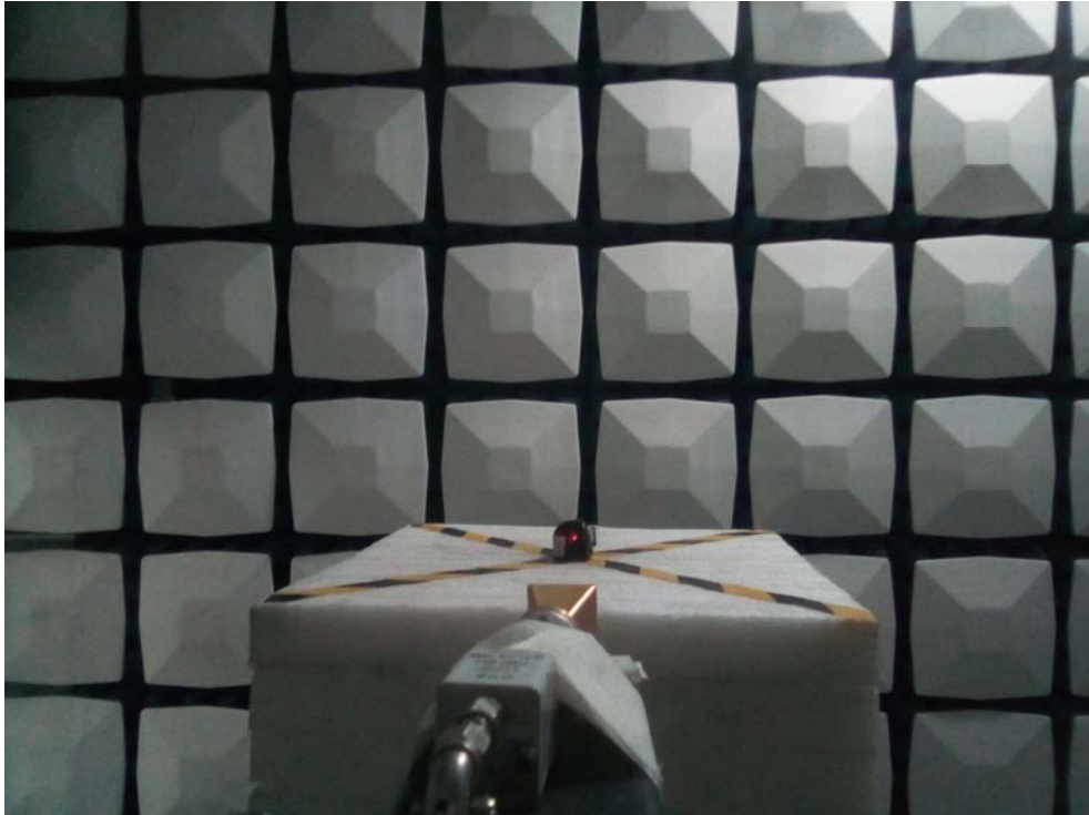
Radiated Emission 26.5GHz-100GHz View(1m distance)
