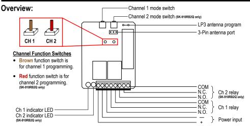
(PC board shown. Remove the front cover of the receiver to access the function switch(es) and terminal block.)
