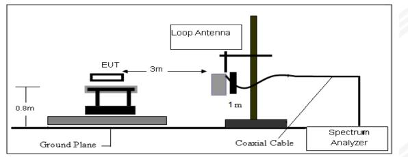
(B) Radiated Emission Test-Up Frequency 30MHz~1GHz
