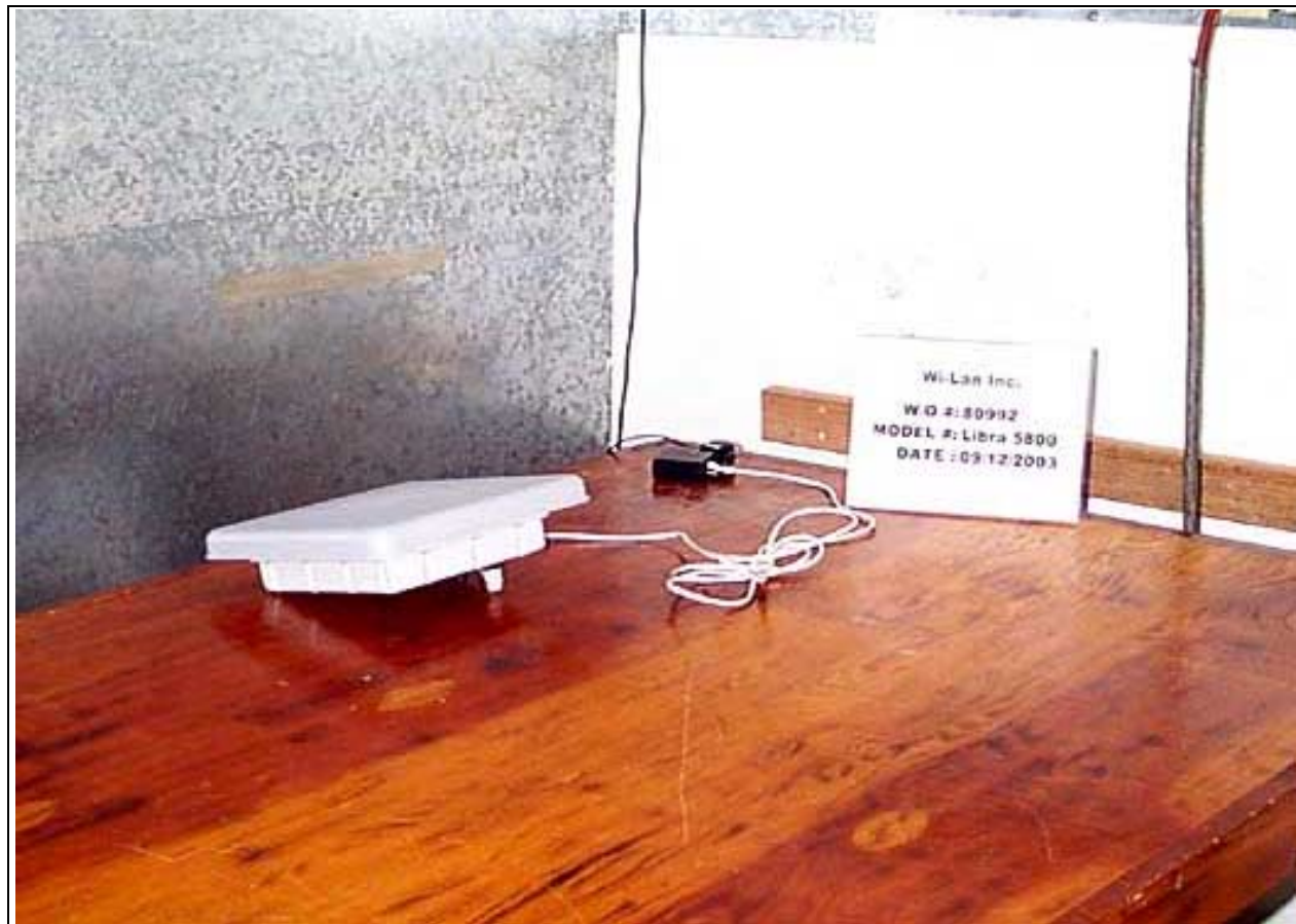
Mains Conducted Emissions - Front View
