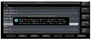
To copy after adjusting the TX equalizer settings, press F5 [COPY] on the TX Equalizer Adjustment screen.
