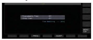
2 Press F3 [PROG] to display the Programmable Timer configuration screen.
