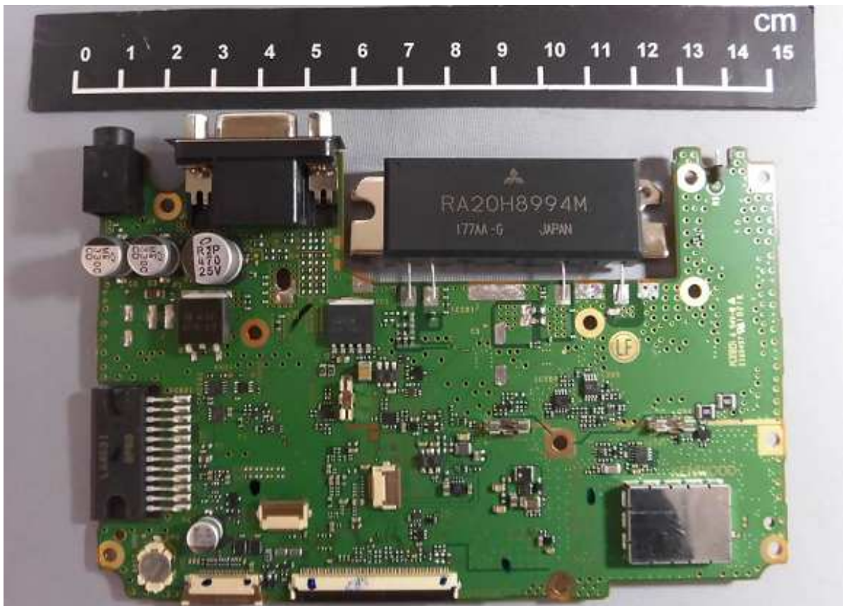
Upper side of TX-RX Unit
