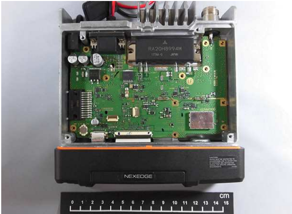
Top Internal View of TX-RX Unit
