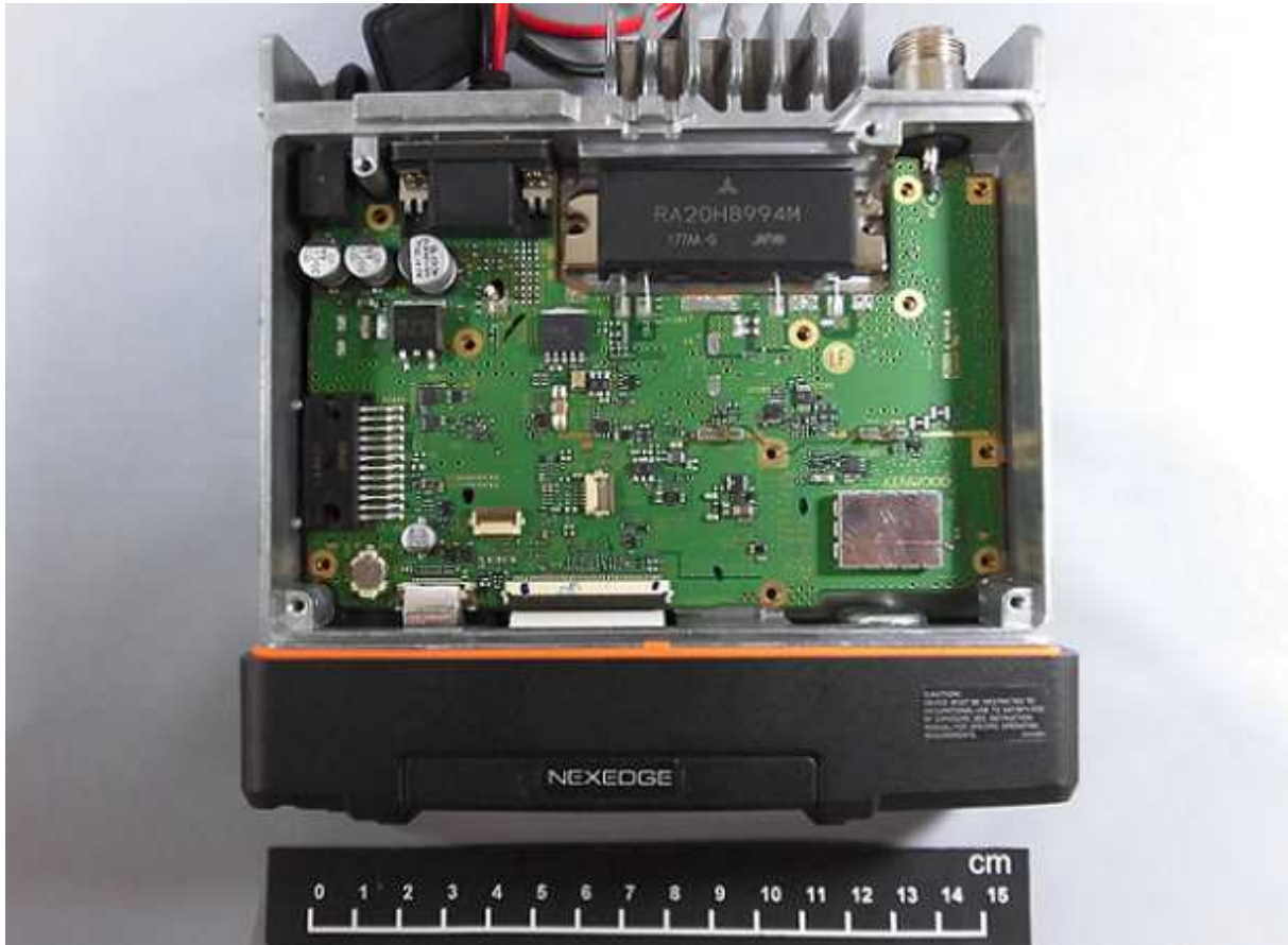
Top Internal View of TX-RX Unit
