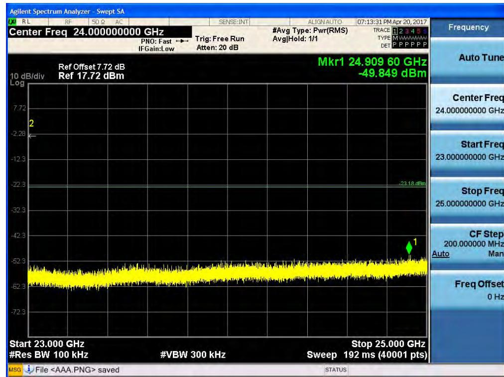
**9.6.2 RADIATED SPURIOUS EMISSIONS****LIMIT : §15.247(d), §15.205, §15.209 / RSS-Gen(Issue 4) Section 8.9, 8.10**
