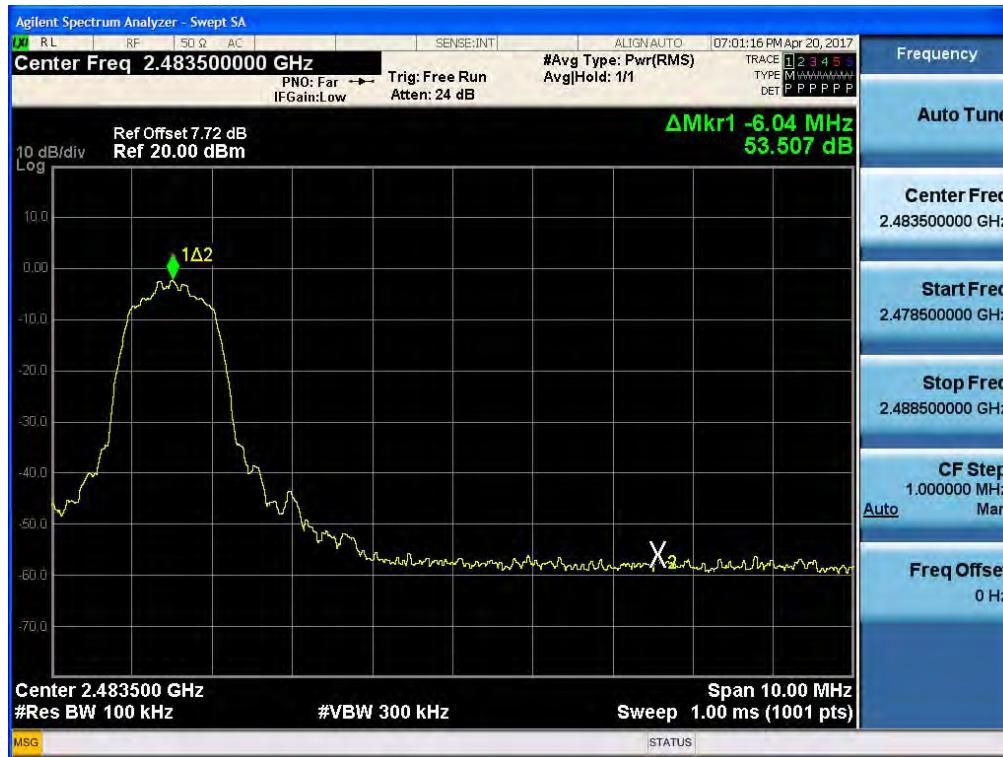
Test Plots with hopping (GFSK)
