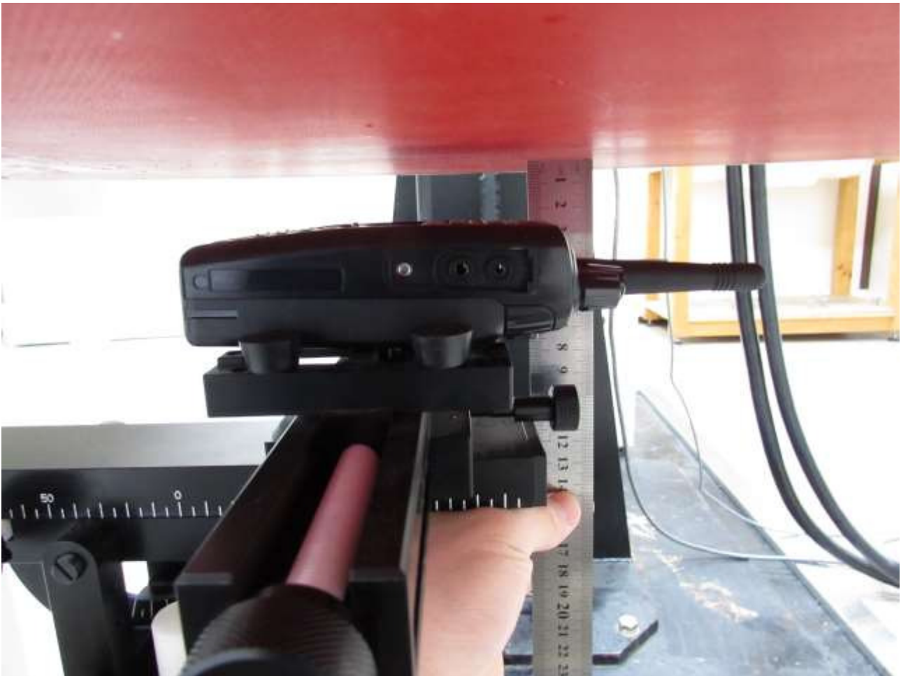
[Distance of 25 mm from the EUT]
