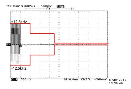
State: High Power / Authorized Bandwidth 11.25 kHz / 8K30F1E/F1D/F7W / 406.15 MHz / PTT:ON -OFF
