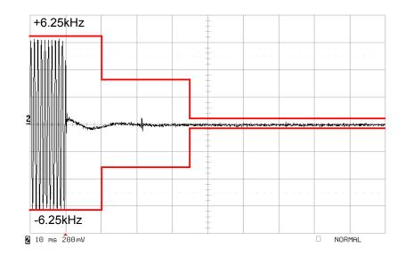
State : High Power / Authorized Bandwidth 6 kHz / 4K00F1E/F1D/F7W / 406.15 MHz / PTT:OFF -ON
