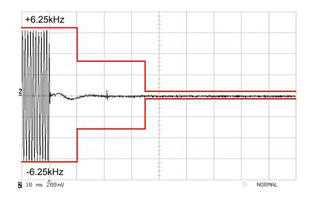
State : High Power / Authorized Bandwidth 6 kHz / 4K00F2D / 438.05 MHz / PTT:OFF -ON
