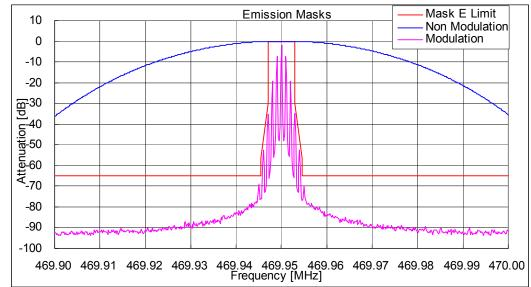
State : High Power / Authorized Bandwidth 6 kHz/ 4K00F2D/ 469.95 MHz FCC Limit : Mask E
