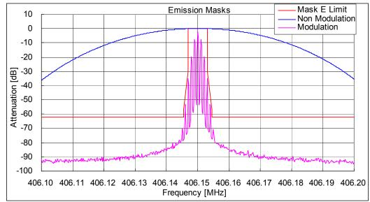
State : Low Power / Authorized Bandwidth 6 kHz/ 4K00F2D/ 406.15 MHz FCC Limit : Mask E
