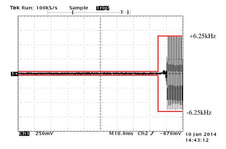
State: High Power / Authorized Bandwidth 6 kHz / 4K00F2D / 150.05 MHz / PTT:OFF -ON
