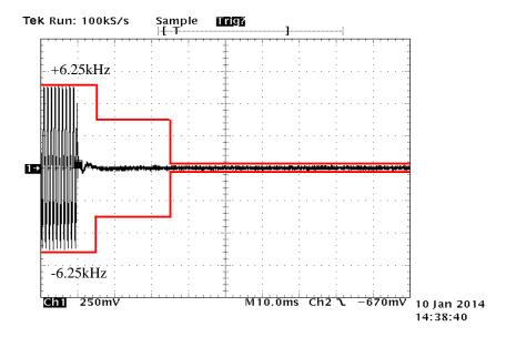
State: High Power / Authorized Bandwidth 6 kHz / 4K00F1E/F1D/F7W / 173.95 MHz / PTT:ON -OFF
