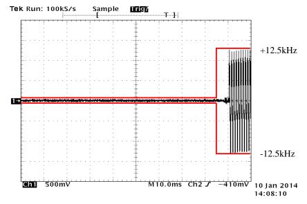
State: High Power / Authorized Bandwidth 6 kHz / 4K00F1E/F1D/F7W / 173.95 MHz / PTT:OFF -ON
