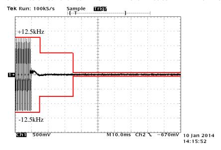
State: High Power / Authorized Bandwidth 11.25 kHz / 11K0F3E / 150.05 MHz / PTT:ON -OFF
