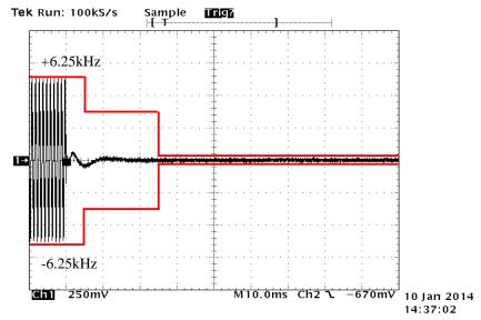
State: High Power / Authorized Bandwidth 6 kHz / 4K00F2D / 150.05 MHz / PTT:ON -OFF
