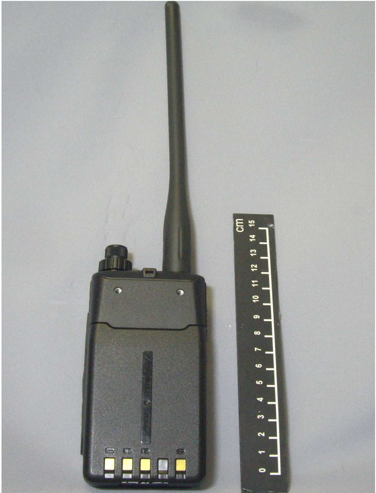
Rear View (with KNB-75L, Antenna )
