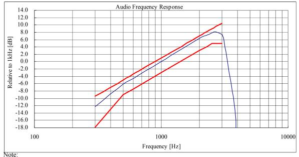
Audio Filter of the above result is substituted with the same structure as Audio Frequency Response. On the transmission condition below 3kHz, Transceiver shows pre-emphasis condition of transmission
