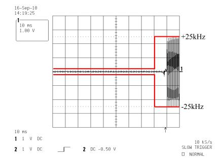
State: High Power / Authorized Bandwidth 11.25 kHz / FM / 450.05 MHz/ PTT:OFF -ON
