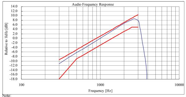
Audio Filter of the above result is substituted with the same structure as Audio Frequency Response. On the transmission condition below 3kHz, Transceiver shows pre-emphasis condition of transmission function.
