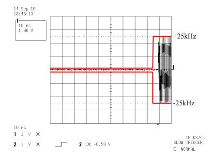
State: High Power / Authorized Bandwidth 11.25 kHz / FM / 150.05 MHz/ PTT:OFF -ON
