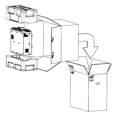
This transceiver is precise and sensitive. To prevent it from being damaged during transportation, the transceiver must be packed with its original packing materials and transported with the front panel facing up. Do not transport the transceiver placed sideways. To prevent injury, transport the transceiver with at least two workers.
