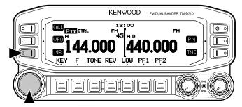
2 Rotate the **Tuning** control to select your desired Memory channel.
