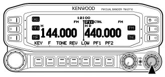
Pressing **[PF2]** allows you to switch the operating band between bands A and B, while maintaining the original band as the transmit band.
