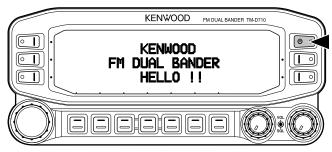
Press the [**b**] switch again to switch the transceiver OFF.
