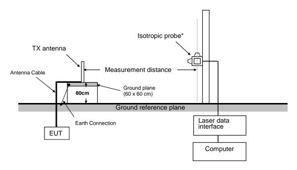
\*: The Isotropic probe position was Vertical orientation from the Ground reference plane from 0.1m to 2m (10cm increments) .
