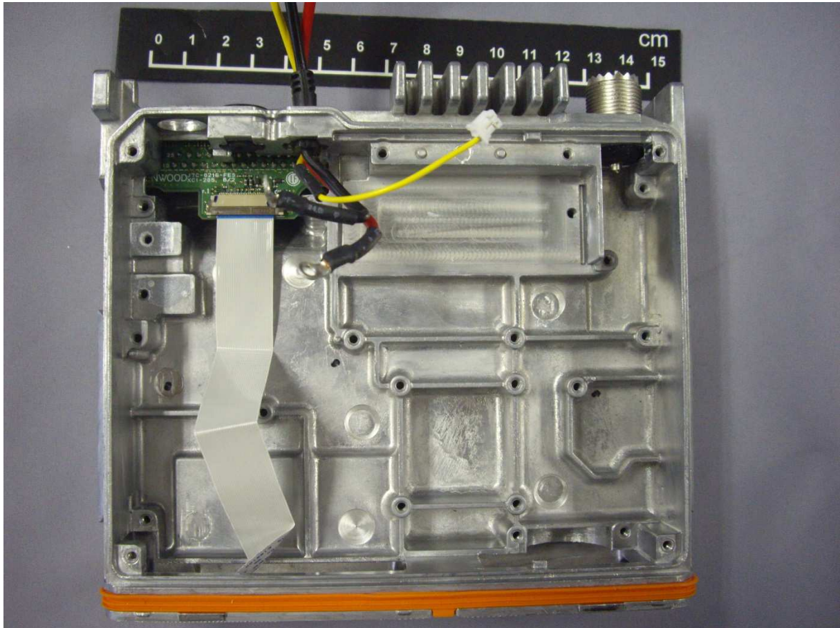
Internal View of D-Sub Unit
