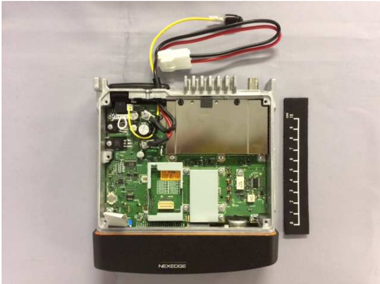
Top Internal View of Main Unit
