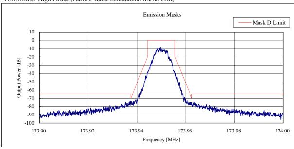
State: 173.95MHz High Power (Wide Band Modulation:4Level FSK)
