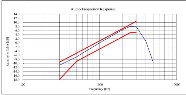
State: 155.05MHz High Power Narrow Band Modulation
