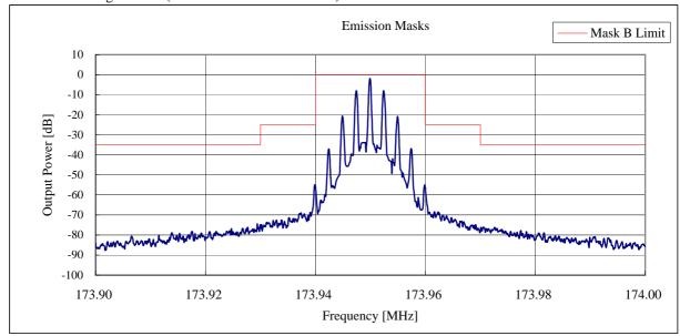
State: 173.95MHz High Power (Narrow Band Modulation:4Level FSK)
