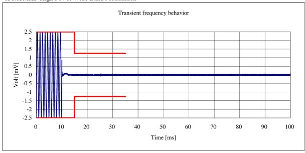
State: 136.05MHz High Power Wide Band Modulation PTT: ON-OFF
