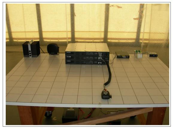
**5.3 Field Strength of Spurious Radiation : Front view** Accordance with TIA-603-C 2.2.12.2
