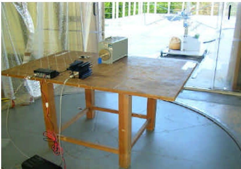
Field Strength of Spurious Radiation : Rear view
