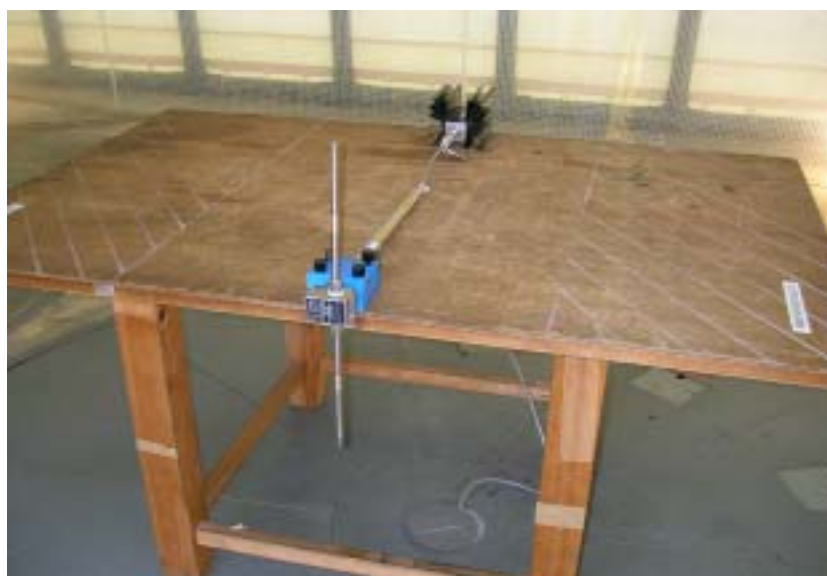
Field Strength of Spurious Radiation (Replace Method)
