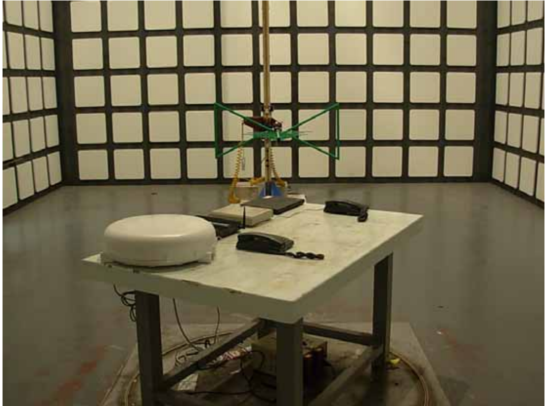
SETUP WITH MAXIMUM DETECTED EMISSION AT HORIZONTAL POLARIZATION (TEST MODE: CH11 (2462MHz) 2MHz)
