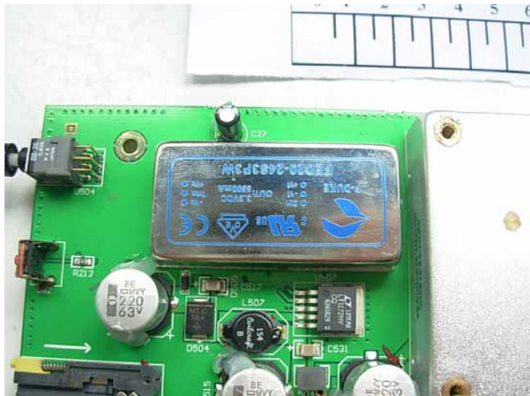
FIGURE 10 LAND MOBILE TERMINAL (M/N: 9350-10) MAIN BOARD – MODULE
