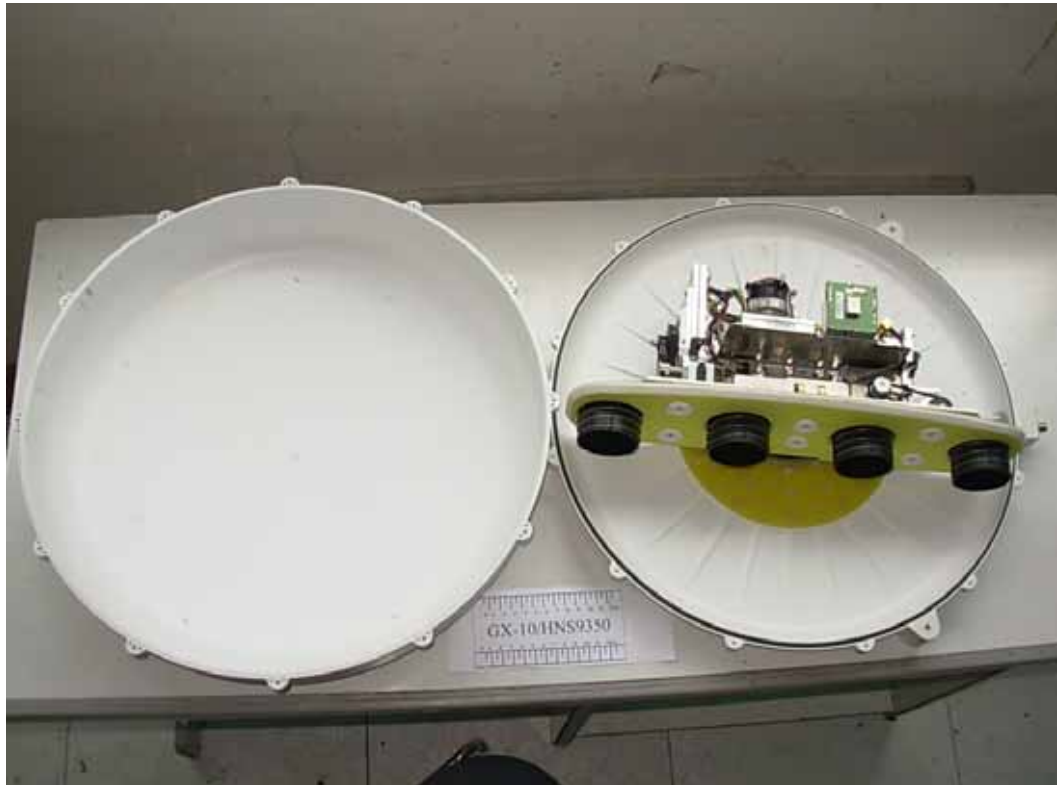
FIGURE 22 LAND MOBILE TERMINAL (M/N: 9350-10) SATELLITE ANTENNA – COVER REMOVED
