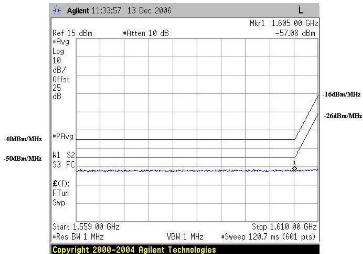
Figure 86. GPS Band Emissions, QPSK 1 Mid Channel
