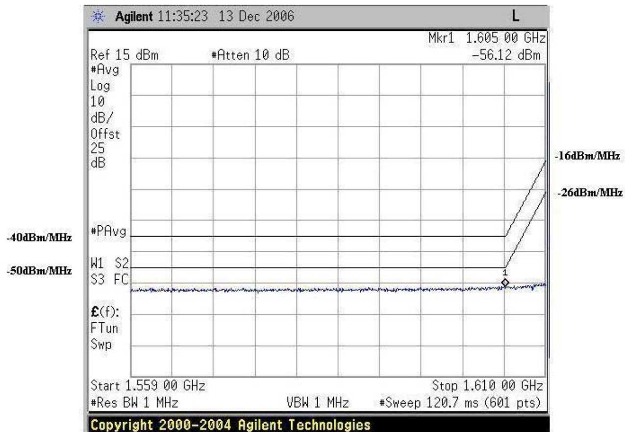
Figure 88. GPS Band Emissions, QPSK 2 Low Channel
