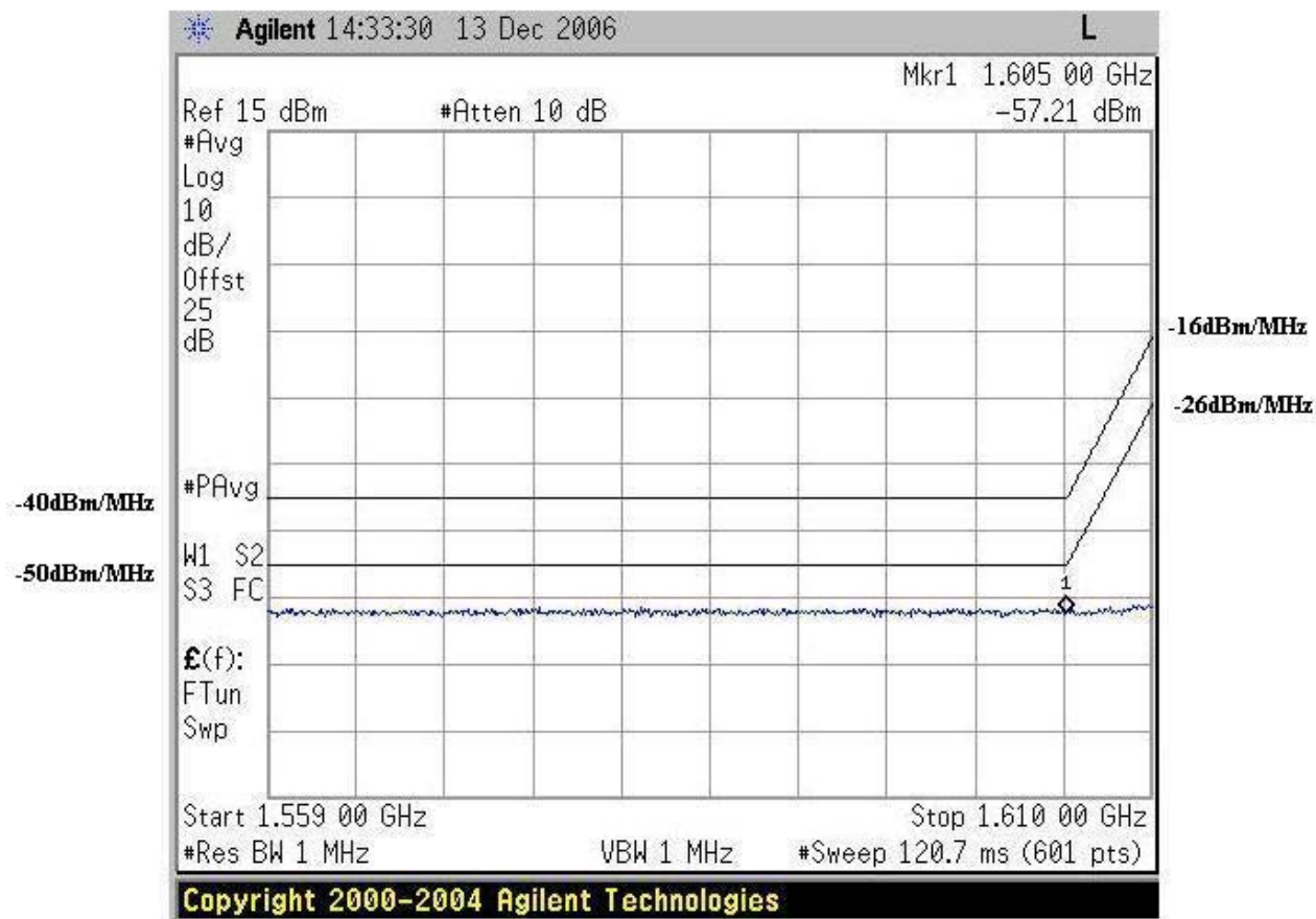
Figure 81. GPS Band Emissions, QAM 4.5 High Channel
