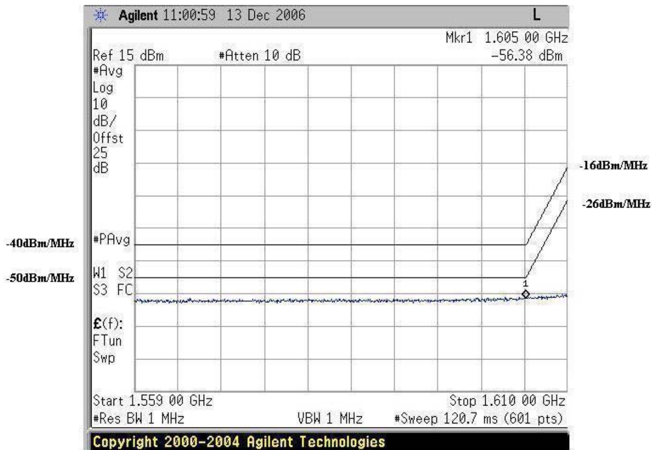
Figure 82. GPS Band Emissions, QPSK 0.5 Low Channel
