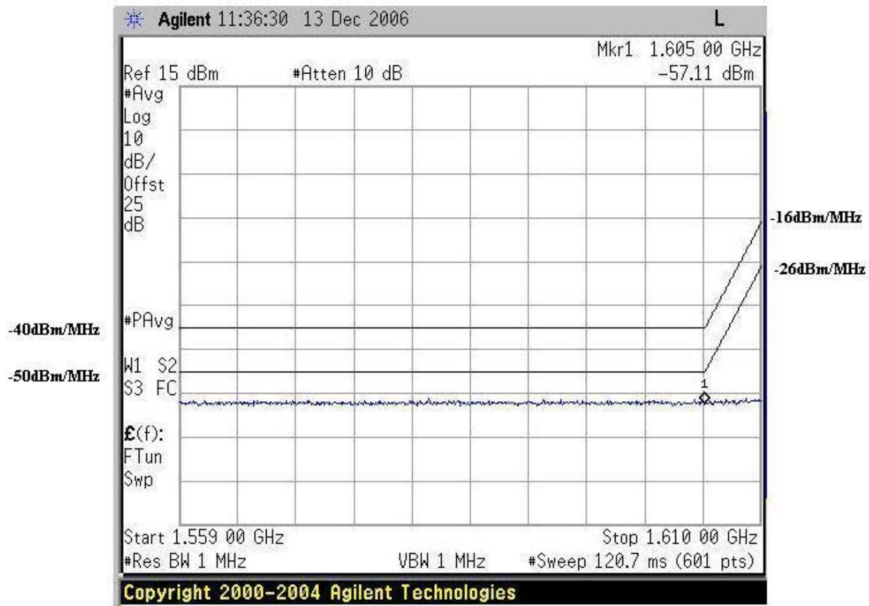
Figure 89. GPS Band Emissions, QPSK 2 Mid Channel
