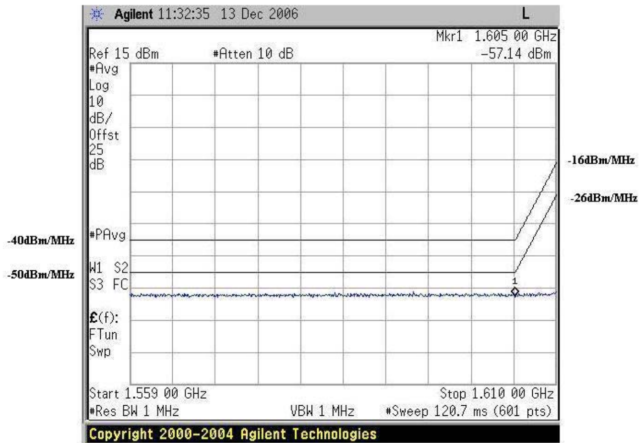
Figure 84. GPS Band Emissions, QPSK 0.5 High Channel
