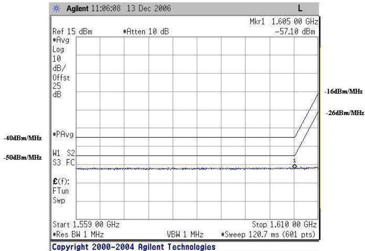
Figure 77. GPS Band Emissions, QAM 2 Mid Channel
