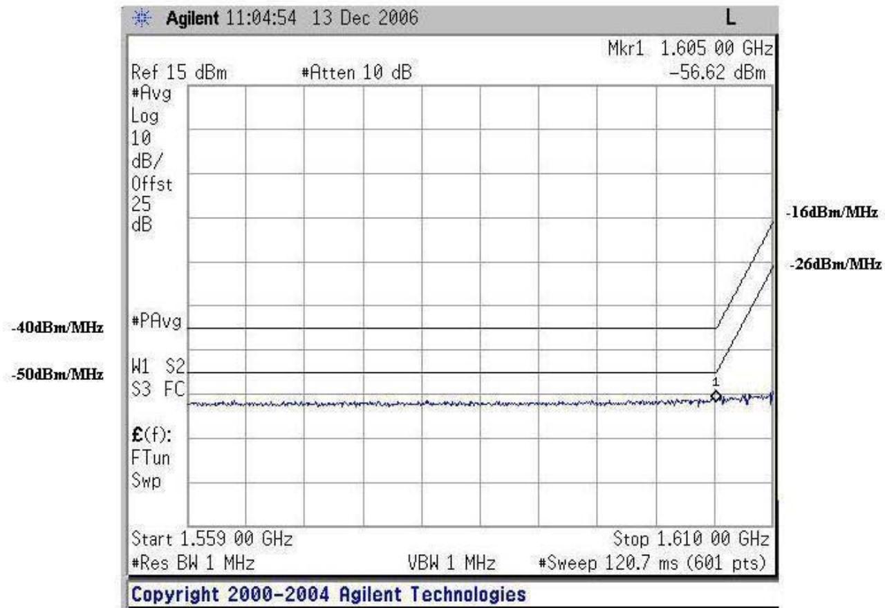
Figure 79. GPS Band Emissions, QAM 4.5 Low Channel
