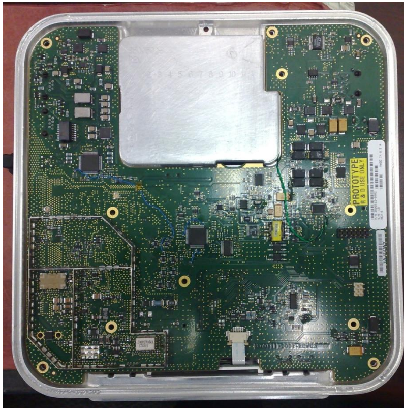
Interface Board – Top side within enclosure
