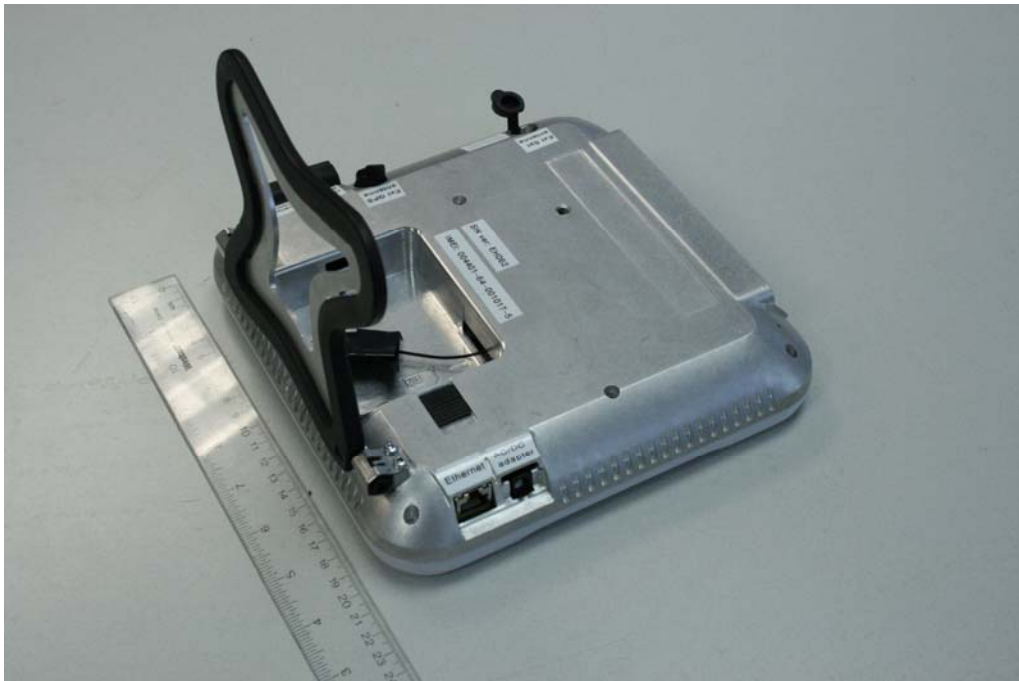
EUT without battery and with antenna test port installed
