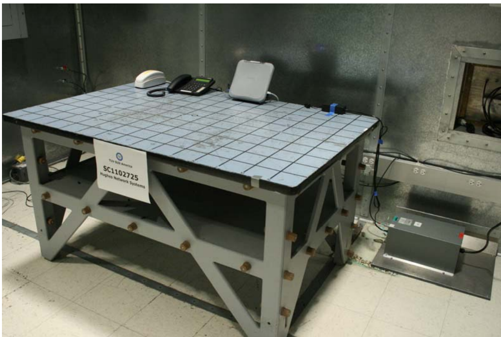
Conducted Emissions Test Setup
