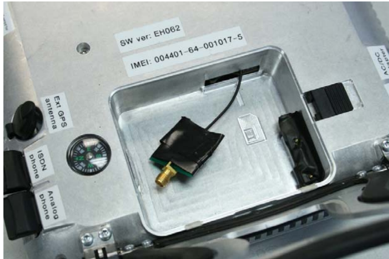
Antenna test port for conducted measurement
