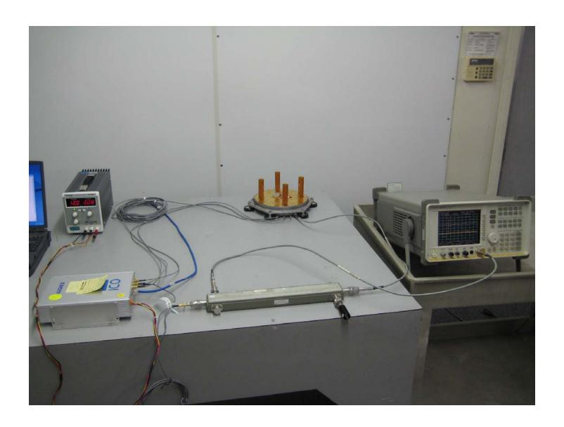
Conducted Emissions at Antenna Terminal Setup
