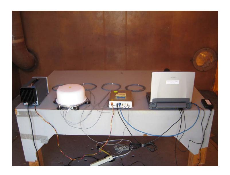
Radiated Emissions Measurement (Rear View) 30-1000MHz
