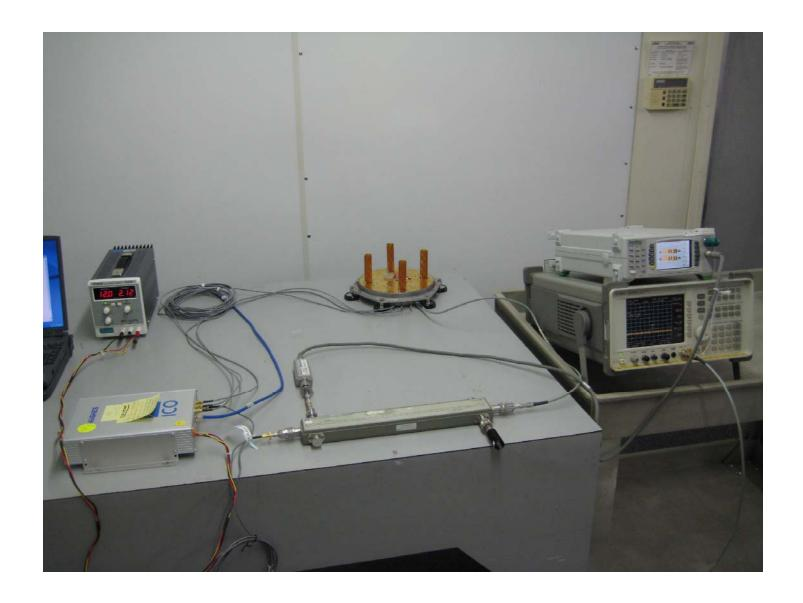
Maximum Peak Output Power Measurement Setup
