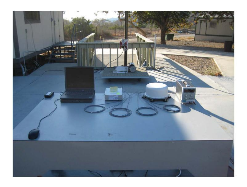
Radiated Emissions Measurement (Front View) 1-18GHz
