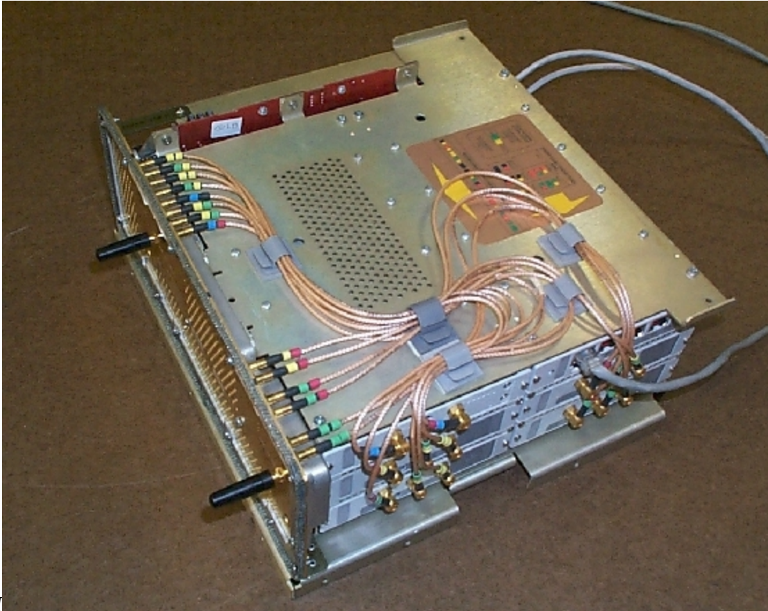
Figure 9.3: Picocell System with All Modules
