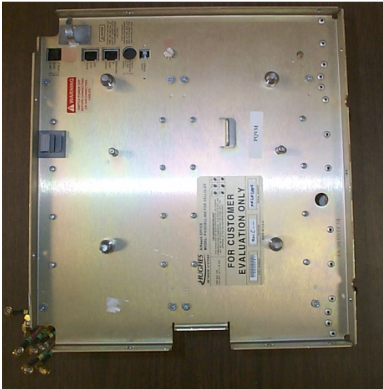
Figure 1.2: 1900 MHz Picocell System Label Area of Placement
