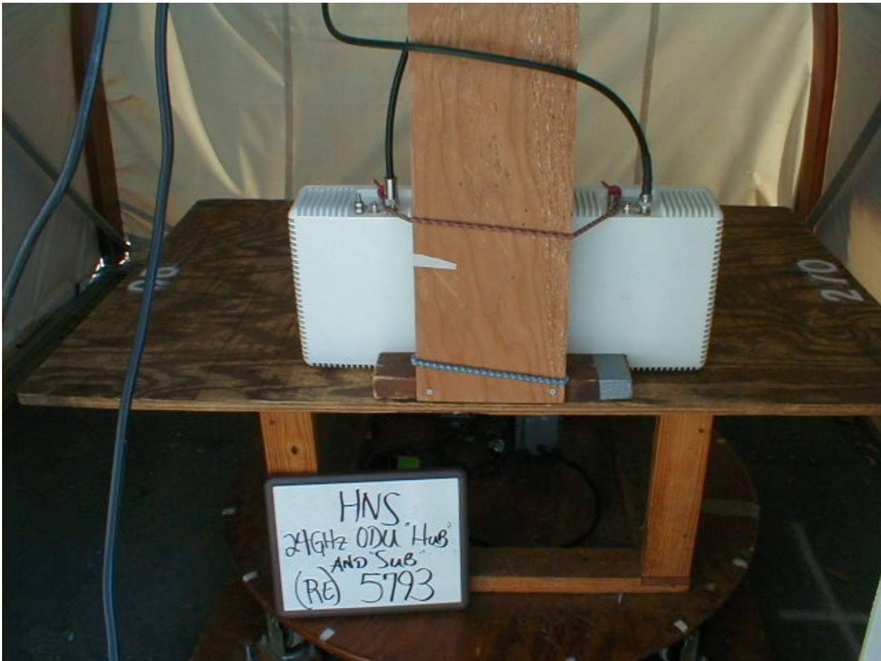
Figure 39 Both Hub and SUB units while doing FCC 15 radiated Emission testing (3m) for class B (Back)
