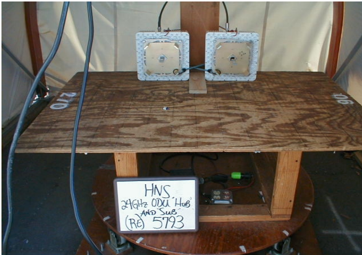
Figure 38 Both Hub and SUB units while doing FCC 15 radiated Emission testing for class B (Front)
