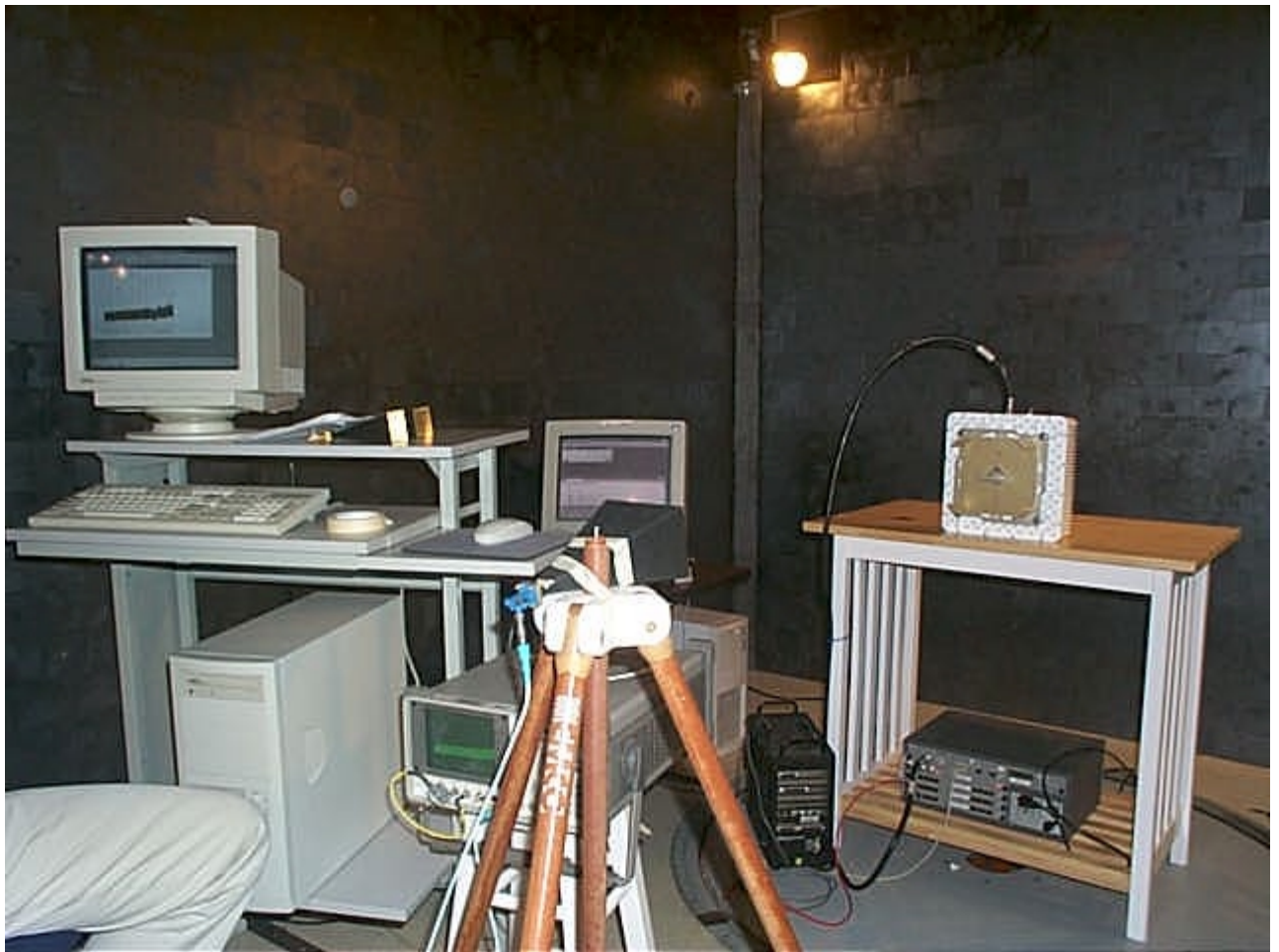
Figure 2 Radiated Spurious Emissions – Test setup
