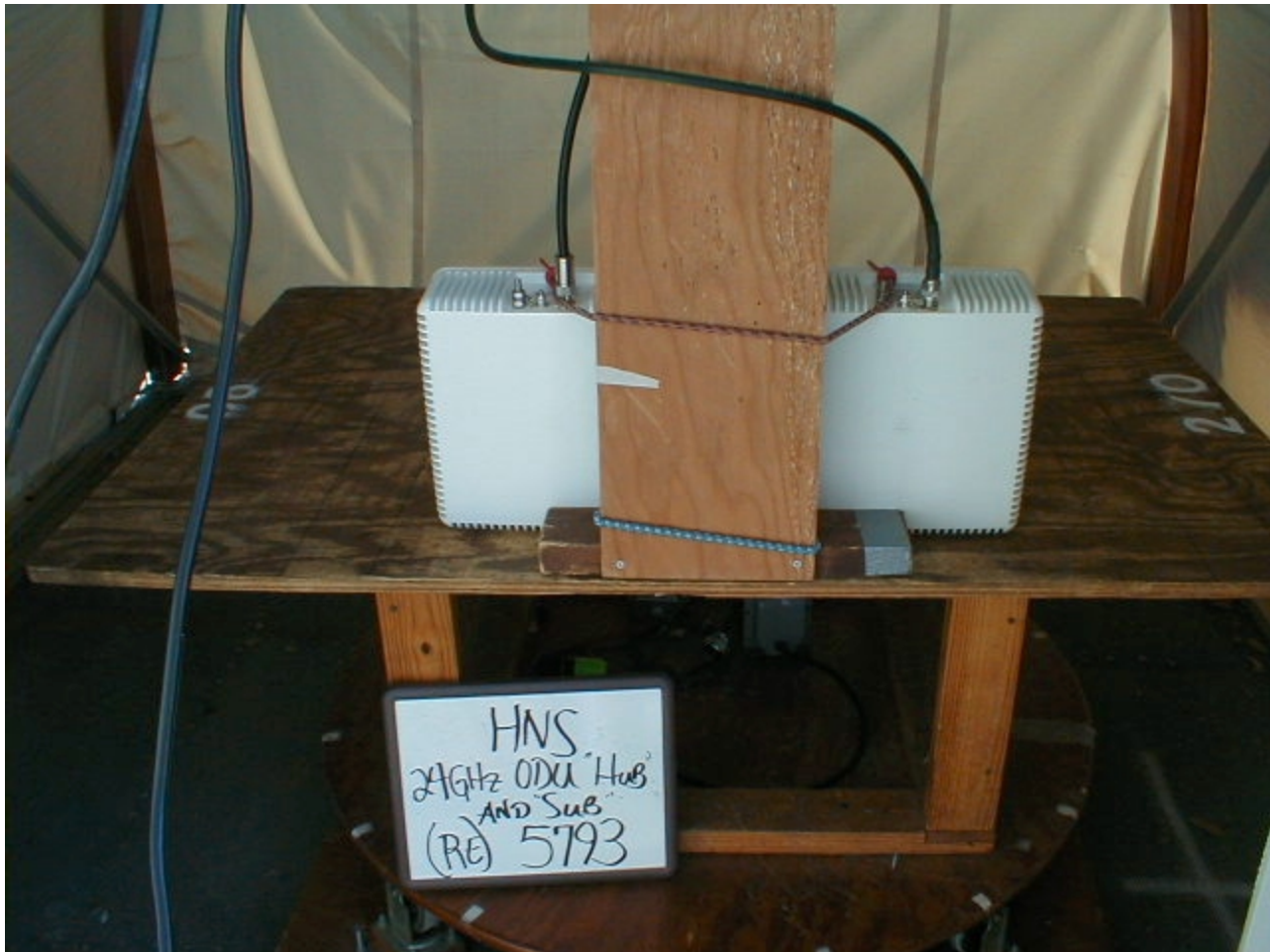
Figure 42 Both Hub an SUB units while doing FCC 15 radiated Emission testing (3m) for class B (Back)
