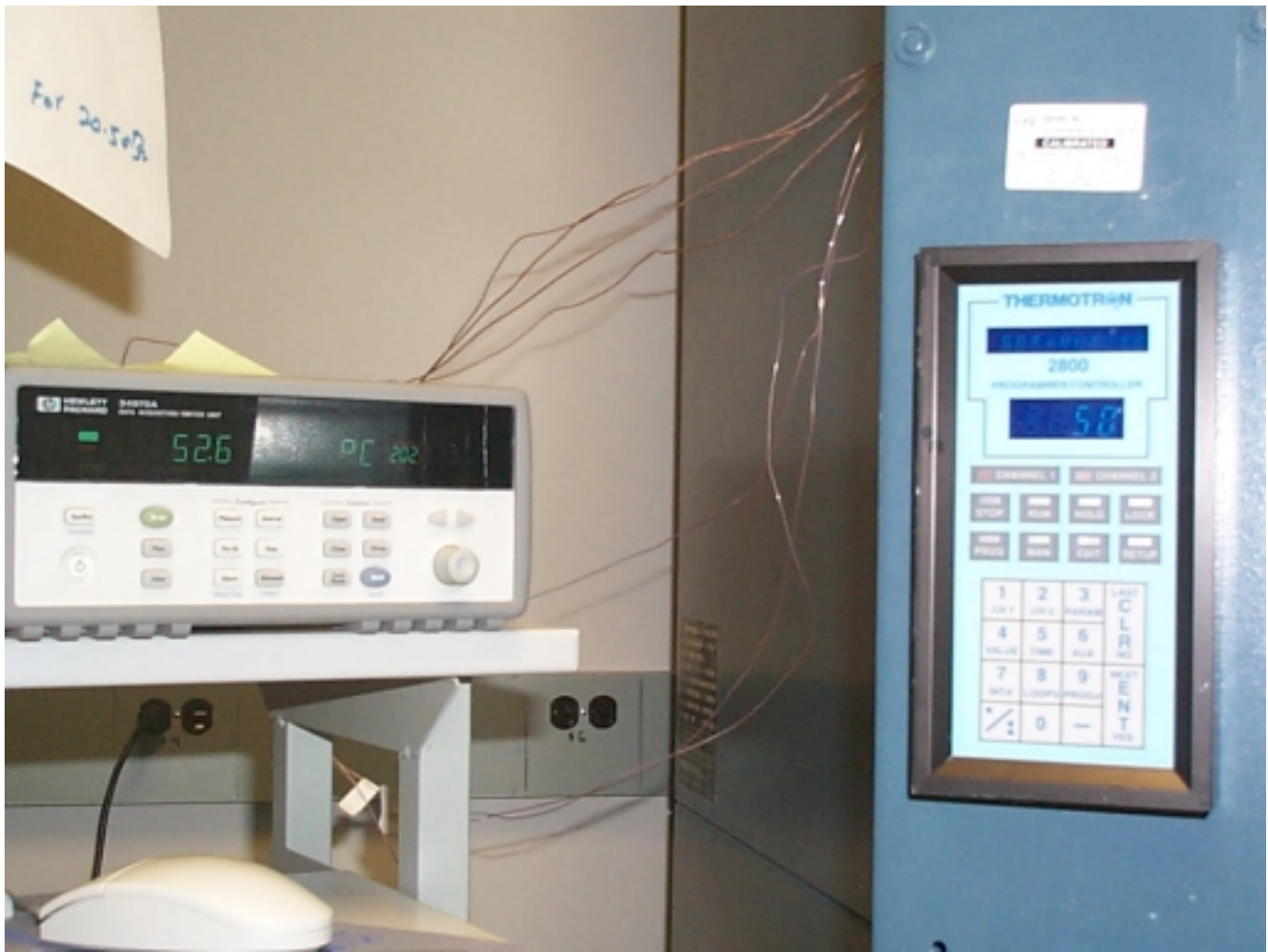
Figure 58: Frequency stability temperature reading acquisition
