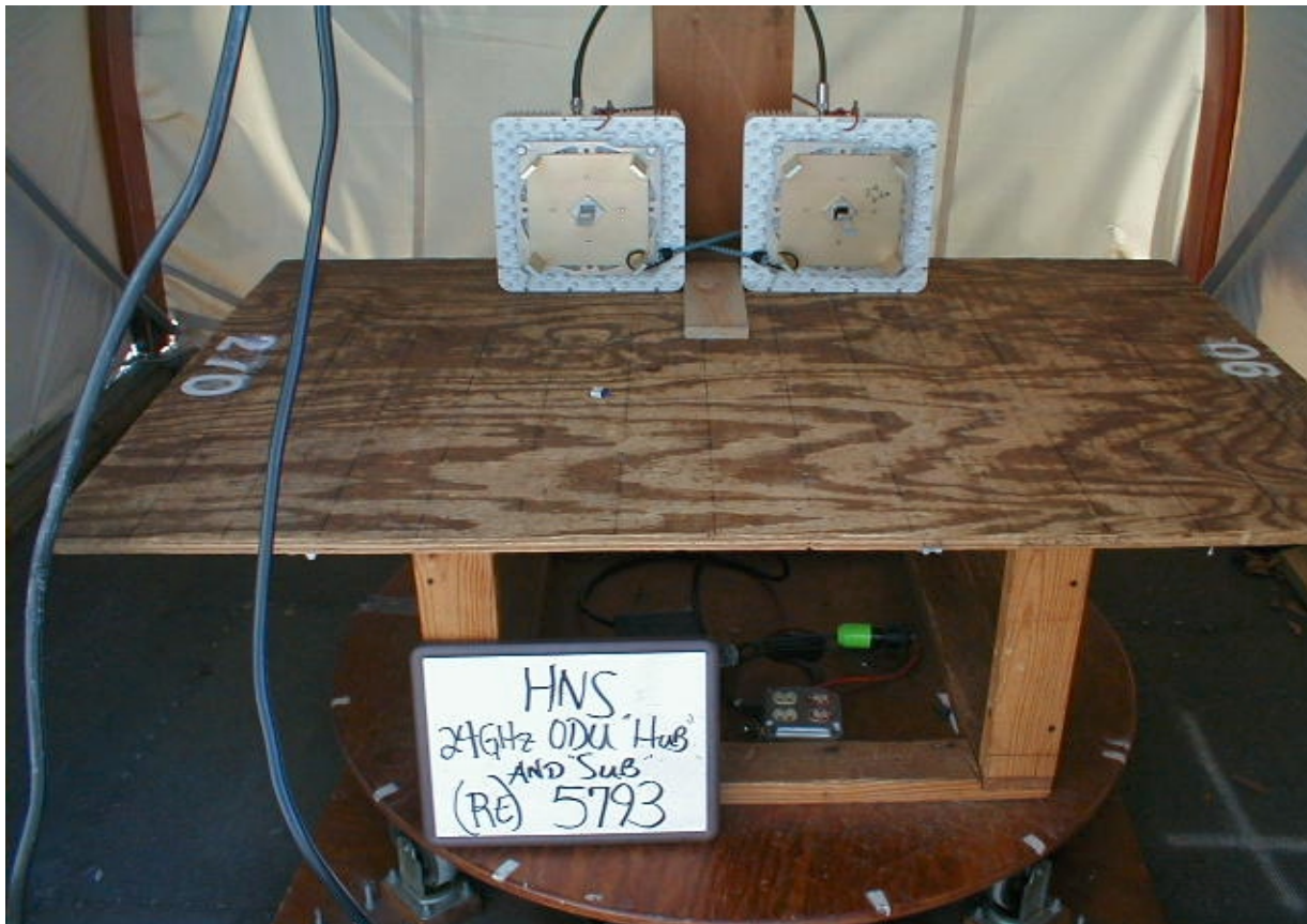
Figure 41 Both Hub and SUB units while doing FCC 15 radiated Emission testing for class B (Front)
