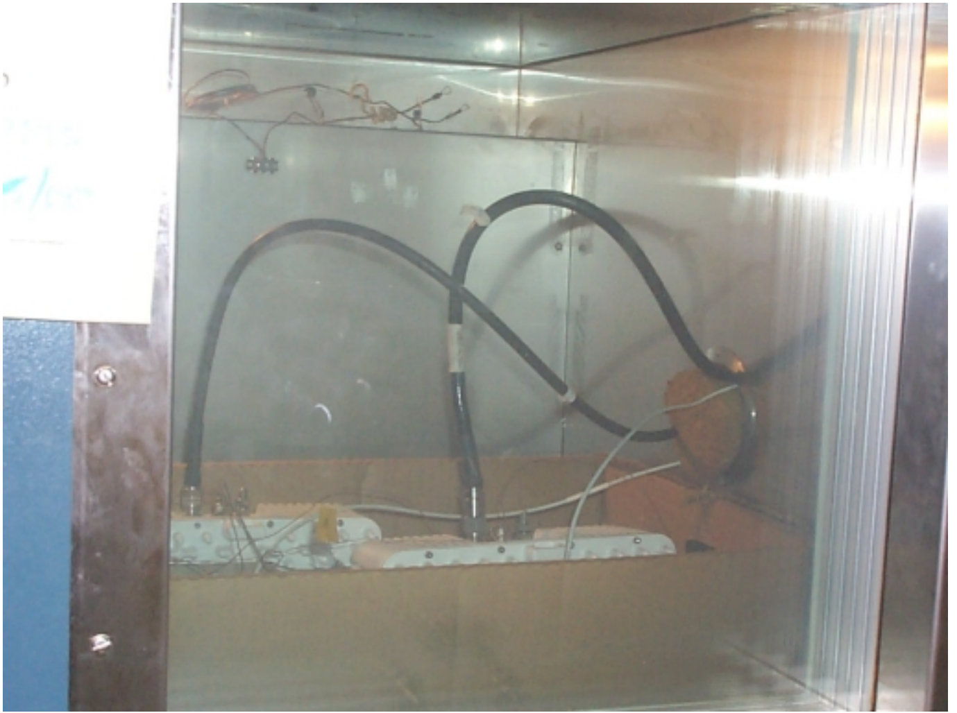
Figure 57: Frequency stability testing EUTs (SUB and HUB) in the Temperature chamber.
