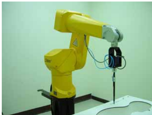
Fig. 5.2 Probe setup on robot
