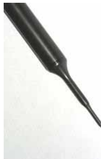
Fig. 5.3 EX3DV3 E-field Probe
