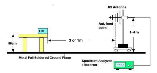
Above 5GHz shall be extrapolated to the specified distance using an extrapolation factor of 20 dB/decade form 3m to 1m.
