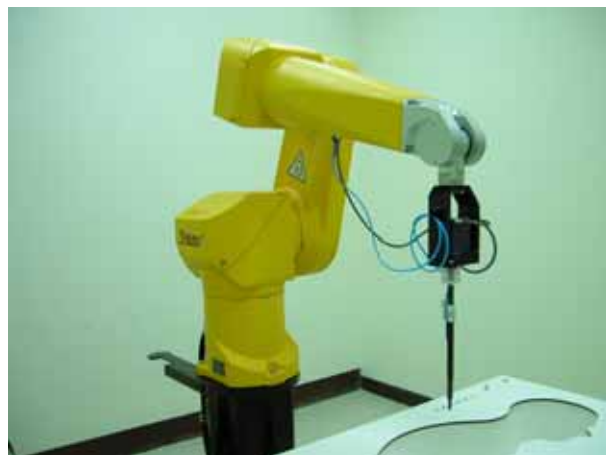
Fig. 5.2 Probe setup on robot
