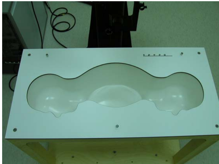
Fig. 5.3 Top view of twin phantom
