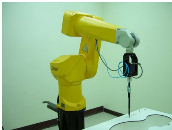
Fig. 5.2 Probe setup on robot
