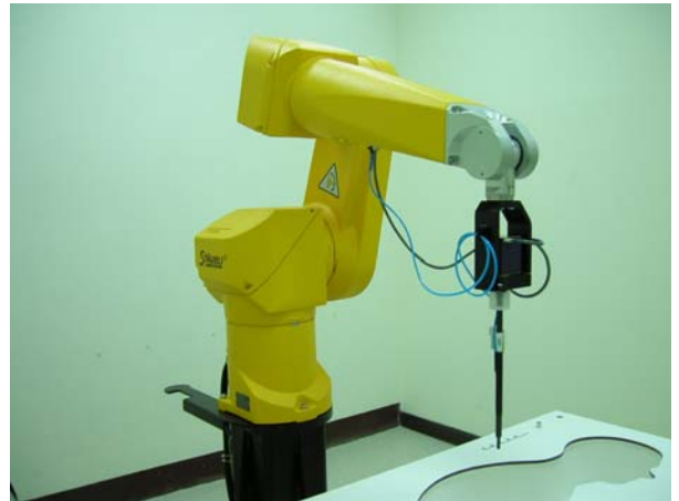
Fig. 5.2 Probe setup on robot
