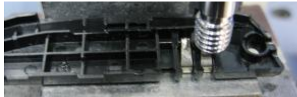
FIGURE 6. Compression Test Method
