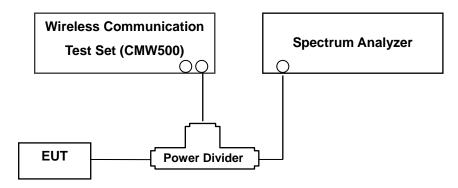
(Configuration of conducted Emission measurement) Test Procedure
