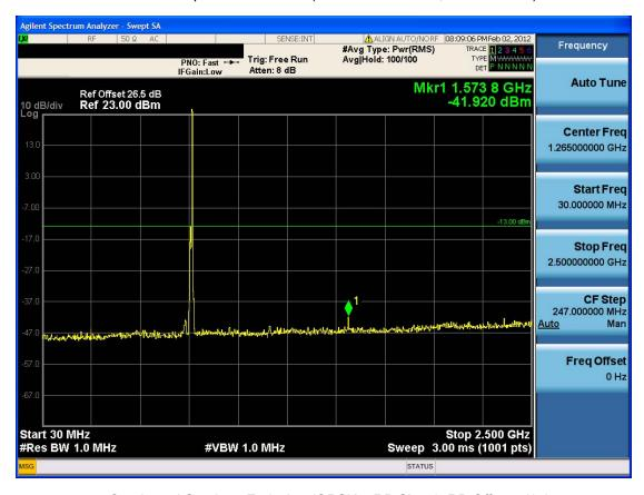
■ Conducted Spurious Emission (QPSK – RB Size 1, RB Offset 49)-2
