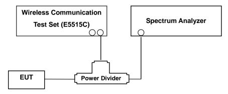
(Configuration of conducted Emission measurement) Test Procedure
